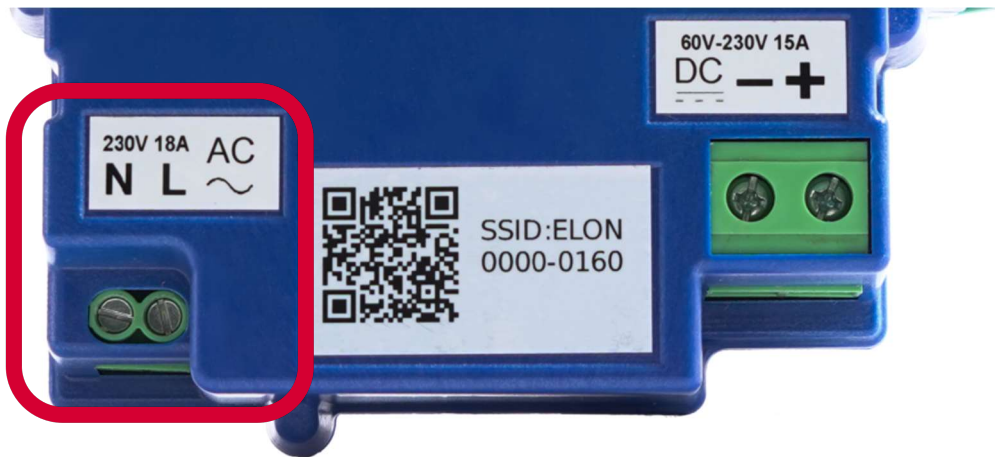
Figure 4.4. STEP 12: The AC screw terminals are located on the left of the Elon Smart Thermostat
