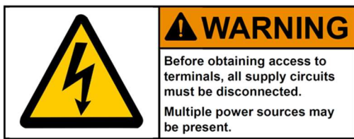
c. Warning – disconnect supply circuits label
